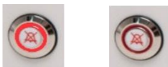
Figure 14.11 Alarm key which indicates the alarm condition
