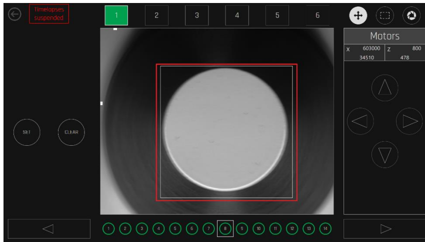
Figure 20.30 Well position inside the marked square limit
