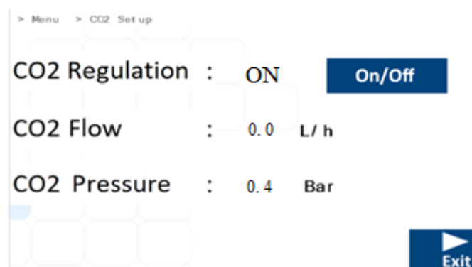
Figure 13.25 CO 2 Setup sub-menu view in the MIRI® TL6 and MIRI® TL12 multiroom IVF incubator
