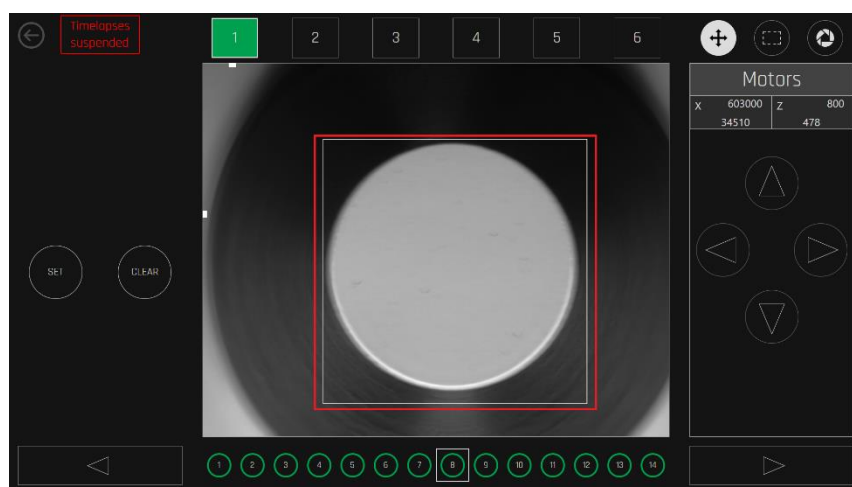
Figure 20.32 Correctly adjusted well's view
